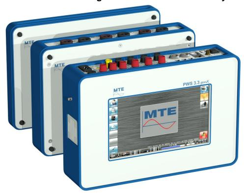
The PWS 3.3 genX is a combination of a Portable Working Standard of class 0.05 % and an IEC 61000-4-30 Class A compatible Power Quality Analyzer with 4 voltage (U1, U2, U3, UN, UPE) and 4 current channels (direct: I1, I2, I3 and via clamp-on CT: IN / IPE Neutral current / Protection Earth current).
